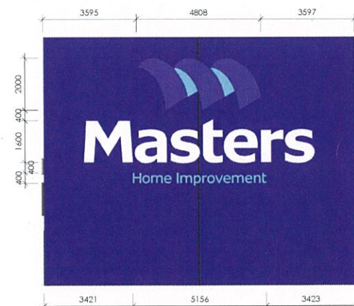
5 MASTERS SIGNAGE 2 DETAILS Scale: 1:100 EXTERNALLY-ILLUMINATED 2000 MM VERTICAL ICON • 4mm ACM PANELING, INDIVIDUAL CUT LETTERS WITH VINYL APPLIED TO FACE • DIRECT FIX
