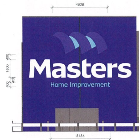
4 MASTERS SIGNAGE 1 DETAILS Scale: 1:100 EXTERNALLY-ILLUMINATED 2000 MM VERTICAL ICON • 4mm ACM PANELING, INDIVIDUAL CUT LETTERS WITH VINYL APPLIED TO FACE • DIRECT FIX
